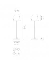
Poldina pro is a battery-operated portable and rechargeable table lamp. It is equipped with: contact charging base and dimmer touch control. Version with metallic leaf finish for indoor use only. Contact charging base included
