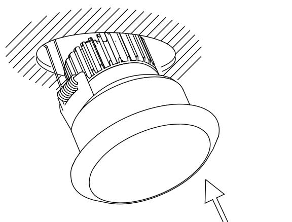
The light source of this luminaire is not replaceable; when the light source reaches its end of life the whole luminaire shall be replaced.
