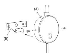
Remove the wall mounting (B) by unscrewing two screws from the lamp body (A).
