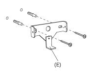
Position the wall mounting and rotate the metal handle (E) to cover the hole on the lamp body. Mount it with two appropriate screws and plugs. Always use correct screws and plugs for the mounting surface.
