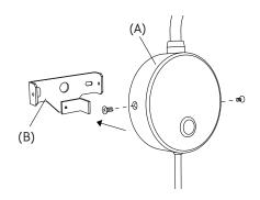
Remove the wall mounting (B) by unscrewing two screws from the lamp body (A).
