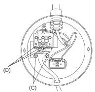
Unscrew the two screws (C) from the back of the lamp housing. Press N, (2), L tabs (D) on terminal strip to pull the cord out.
