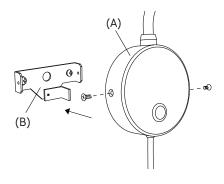
Attach the lamp body back to the wall mounting.
