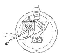
4. Connect the electrical cord with the terminal strip.
