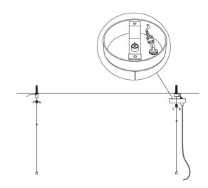
Fasten the wires (Part I and Part J) onto the lampshade (Part A).
