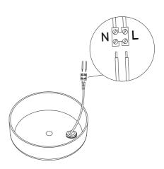
8 Mount wire (Part I) and ceiling cup (Part E) to the bracket (Part F) using the wire lock (Part G).
