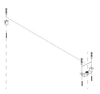
6 Pull the cable that is attached to the lampshade (Part A) through the ceiling cup (Part E).
