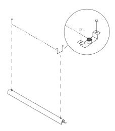
3 Drill the holes and insert plugs (Part C).
