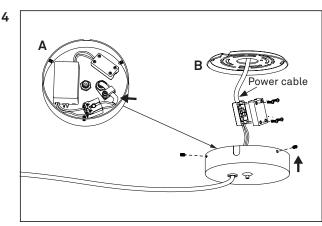
**A:** After stripping the cable, connect the lead with text to the positive and the other lead to the negative wire from the driver.
