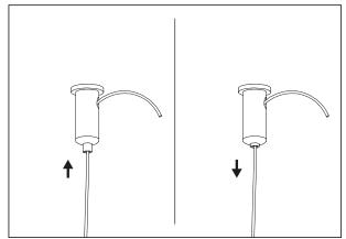
Use the wire lock on the canopy and the ceiling to adjust the lamp to its final position. It is recommended to use a spirit level.
