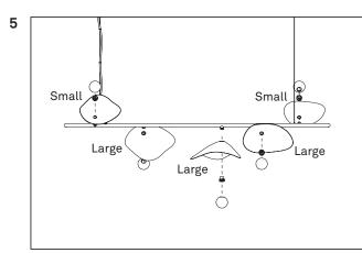
Attach the shades by placing them over the threaded base and lock them in place by screwing a light source on.
