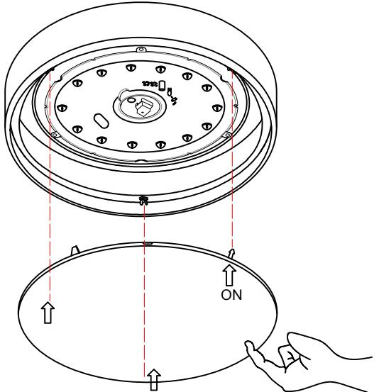
position the lampshade against the spring, lighly press the spring in 3 positions and fix the lampshade in the chassis
