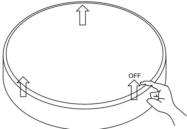
lighty press the spring in 3 positions to lift the lampshade off the chassis
