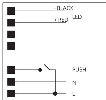
1-10 V DIMM wiring diagram
