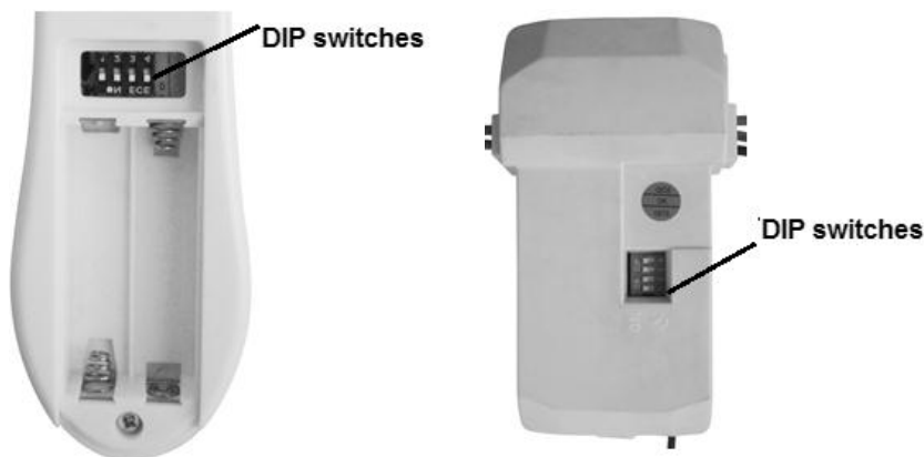
Fig. 8 Remote battery compartment
