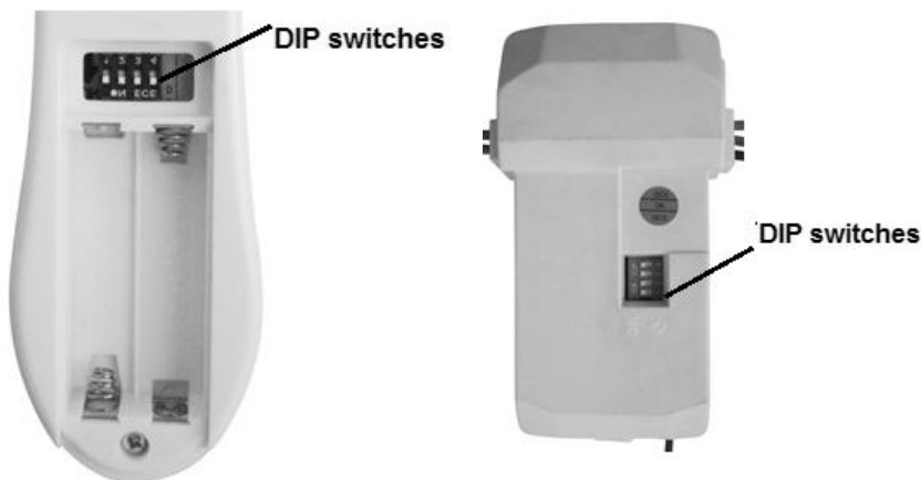
Fig. 8 Remote battery compartment
