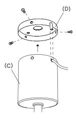
4. Attach the lamp body back to the wall mounting. Align the cable on the lamp body with groove on the ceiling mounting.
