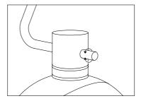
Rotate the switch for turning ON-OFF or dimming the lamp.
