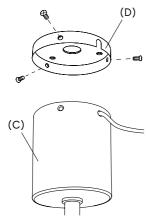
2. Remove the Ceiling mounting (D) by unscrewing three screws from the lamp body (C).
