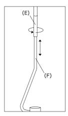
Tighten the shaft. NEVER rotate lamp body around its axis.
