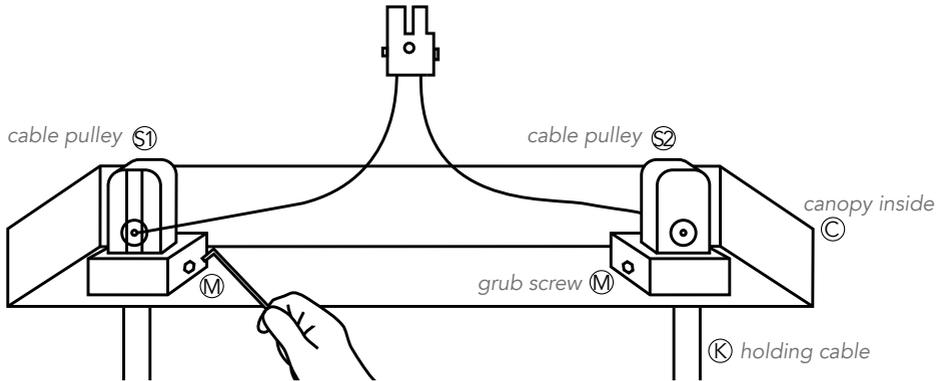
Because wood is a natural product, each piece of wood can vary in density. The weight of every HerzBlut lamp body (1) could be different. The counter weight (F) is set up for an average weight. When the lamp body (1) heavier is as the counter weight the "extra weight" has to be counter balanced.
