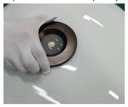
Step 2: separate the round plate and loosen screws on plastic ring with screw driver. Take off the plastic ring.
