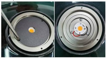
Step 4: Loosen the small screws on white plastic LED holder by screw driver and take it off.
