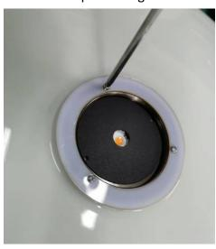
Step 3: Loosen the small screws on black round plate by screw driver and then take off this plate.
