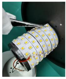
Step 9: Fix a new connection wire to the light source by using electric iron. Take care of the LEDs during this step, do not touch them.
