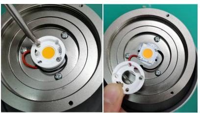
Step 5: Remove the 2 wires from the LED board by using electric iron. Take care of the LEDs during this step, do not touch them. Then first LED part is removed from the lamp.
