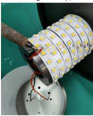
Step 8: Peel off LED with sharp tool, for example tweezers or screw driver . Take care of the LEDs during this step, do not touch them.
