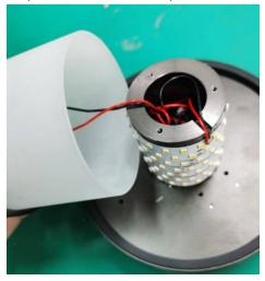
Step 7: Remove the 2 wires from the LED board by using electric iron. Take care of the LEDs during this step, do not touch them.
