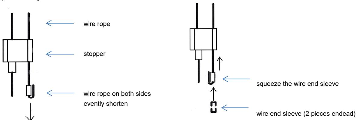
Pull the wire rope down out from the stopper
