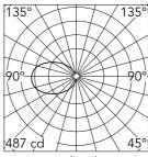
Luminous flux luminaire 551 lm
