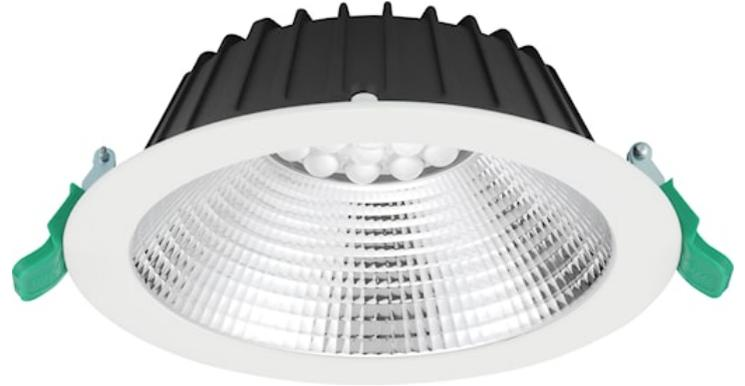
Insaver is a ceiling recessed LED downlight (IP44 from the front), Die-cast aluminium body, loop in loop out connector for quick installation, Dimmable DALI driver of TRIDONIC (LCA 17W 250–700mA one4all SR PRE 28000670), 13W; 1700lm; 131lm/W; 4000K; UGR <19 with shallow product depth 60mm. Meets TP(a) requirements.
