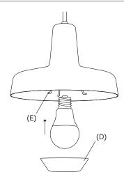
5. To insert the light bulb, release the undershade (D) by pressing three undershade bracket (E) inwards.
