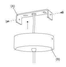
4. Attach the lamp body back to the ceiling mounting.
