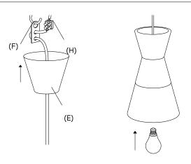
Hang the cable adjuster on the ceiling hook (not included).
