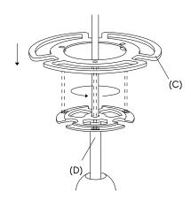
(!) If included, pull the large ring (C) through the cable set (D). Position hooks above the holes and turn counterclockwise to secure.
