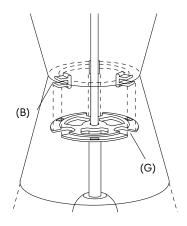
4. Ensure the clips are positioned between the cutouts (G) of the ring in order for the lamp to be balanced.
