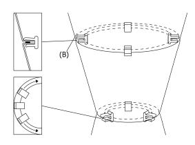
2. Connect the elements with clips (B) so the longer side of the clip is facing wider element. Insert other clips next to the first one and slide at equal distance. For smaller elements use 3, for bigger 4 clips.
