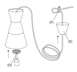
3. Pull the cable set through the lamp. Afterwards, pull the cable through the ceiling cup (E) and cable adjuster (F).
