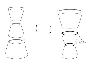
1. Set elements in order then turn them. Start by assembling top two elements first. Do not remove sealing rings (A).
