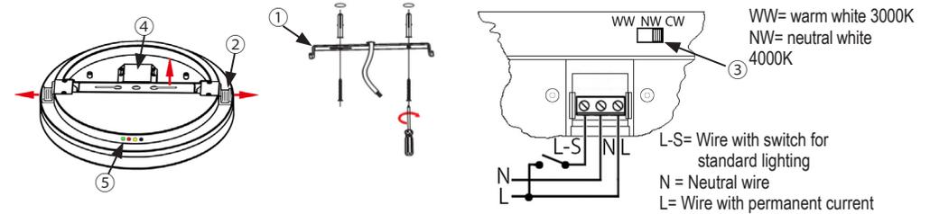
1. Remove the ceiling bracket ① from the light (pull the spring lock ② outwards).
