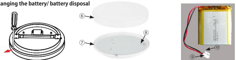
1. Use a flat screwdriver to carefully pry the hood ⑥ off the base plate ⑦.
