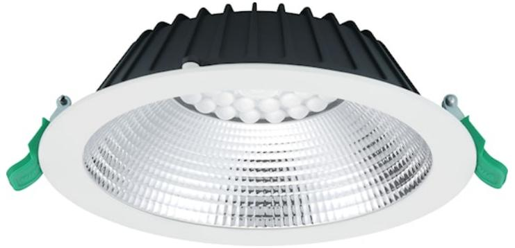
Insaver is a ceiling recessed LED downlight (IP44 from the front), Die-cast aluminium body, loop in loop out connector for quick installation, Non dimmable LED driver, 20W; 2500lm; 125lm/W; 4000K; UGR <19 with shallow product depth 60mm. Meets TP(a) requirements.
