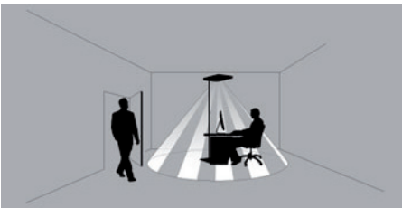
Fig. 17: Sensing range PIR sensor.
