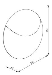
Voltage (V): 220-240 Volt IP degree: IP54 Class (Class 1, Class 2, Class 3): Class 1 (Earth contact)
