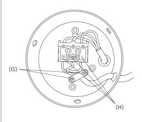
Unfasten the two screws (G) from the back of the lamp housing. Press N, ⊕, L tabs (H) on terminal strip to pull the cable out.
