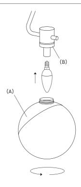
7. Insert the light bulb then gently mount the diffuser screwing it back to the metal ring.
