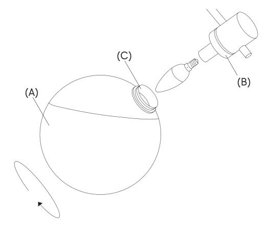
Unscrew the sphere shade diffuser (A) while holding the metal ring (B). Make sure that the bulb diameter is less than 36 mm, so it could fit inside the metal part (C).
