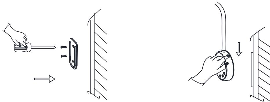
Method 2: Fix the plastic glue nail on the wall, then fix the support plate on the wall with screws, and slide the lamp onto the support plate
