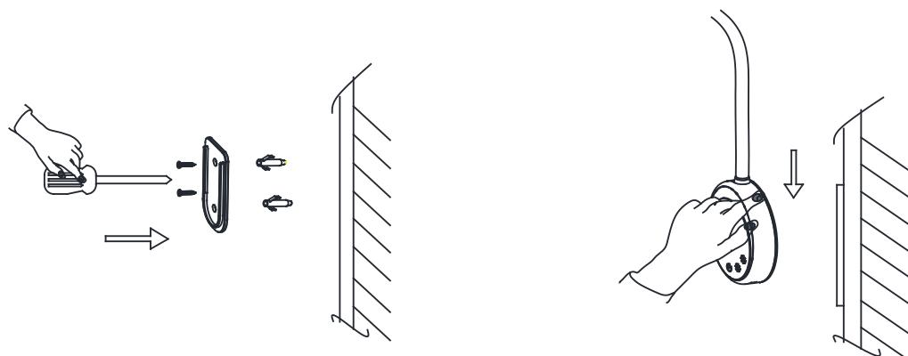
Method 3: stick the self adhesive tape on the surface of the support plate, fix it on the wall, and slide the lamp base onto the support plate
