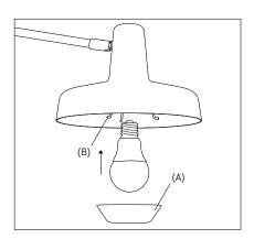
To insert the light bulb, release the undershade (A) by pressing the undershade brackets (B) inwards.
