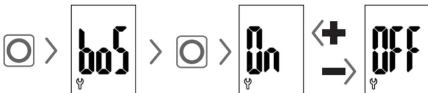
The boost function enables the room to be heated for a short time and is automatically deactivated after 15 minutes.
