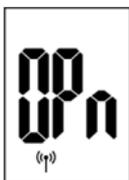
If an open window is detected by an external DuoFern window/door contact, this message (**OPn**) appears for the duration of the process.
