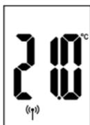
The normal display appears with the set target temperature after a successful installation run.
