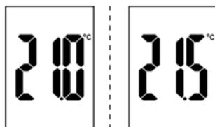
You can adjust the desired target temperature in 0.5 °C steps by briefly pressing the button.
