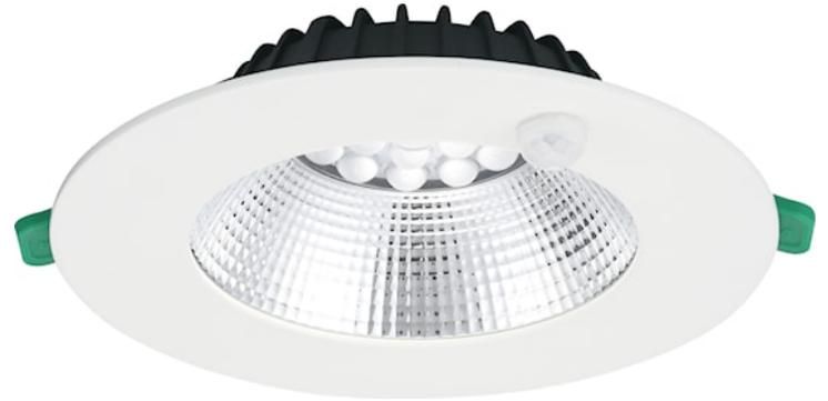
Insaver is a ceiling recessed LED downlight (IP44 from the front), with integrated PIR sensor with time ( up to 8 mins ) and daylight lux level settings. Die-cast aluminium body, loop in loop out connector for quick installation, Non dimmable LED driver, 9.5W; 1200lm; 126lm/W; 4000K; UGR <19 with shallow product depth 50mm. Meets TP(a) requirements.
