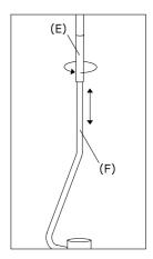
Tighten the shaft. NEVER rotate lamp body around its axis.
