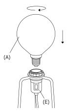
3. Screw the glass diffuser (A) onto the lampholder.
