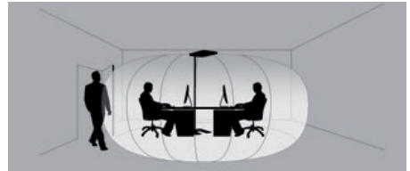
Fig. 11: Detection range of the HFMD.
