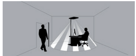
Fig. 12: Detection range of the PIR sensor.
