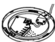
The area in front of the bayonet lock (dotted in the picture) is NOT an installation area. This means that no wires may be routed there. The wires could be injured by the mechanical movement of the closure.
