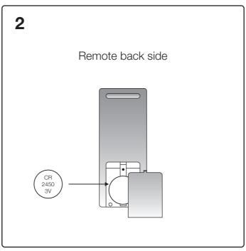
Remove the battery cap and insert 1 x CR 2450 3V battery.
