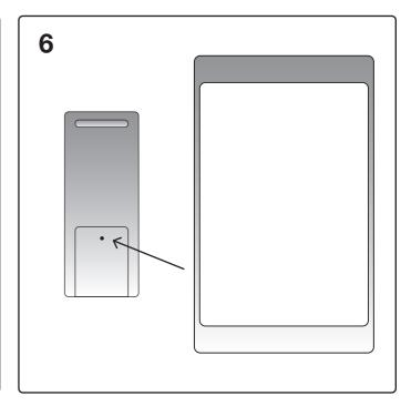
Click on "settings". To enter the settings you need to press and hold the setup button with a pointed object on the back of the Remote Control for 5 seconds. The '1' in the upper corner will start flashing blue.
