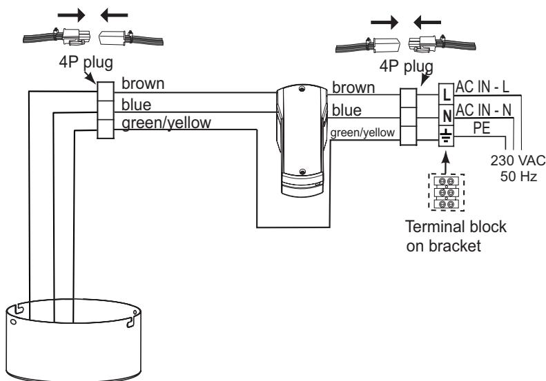
Connect the plugs as shown in the picture and connect the mains voltage at the terminal block.
