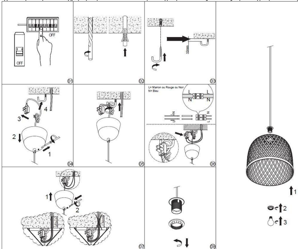
**Any electrical connection should be made only by a qualified electrician.**
