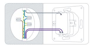
Remember which line goes where, for example by marking it with adhesive tape. Then disconnect the existing wiring and remove your old light switch.
