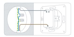
Remember which line is connected to the input on your old light switch (L), for example by marking it with adhesive tape. Then disconnect the existing wiring and remove your old light switch.
