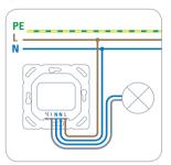
Eve Light Switch does not require a connection to a protective conductor / ground wire (PE, usually green yellow).
