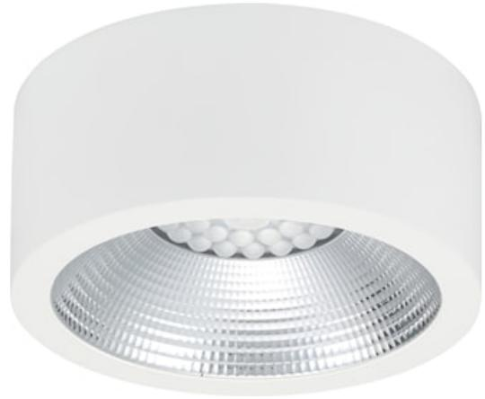
Insaver is a surface mounted LED downlight, Die-cast aluminium body, loop in loop out connector for quick installation, Non dimmable LED driver, 20W; 2500lm; 125lm/W; 4000K; UGR <19 with height of 95 mm. Meets TP(a) requirements.
