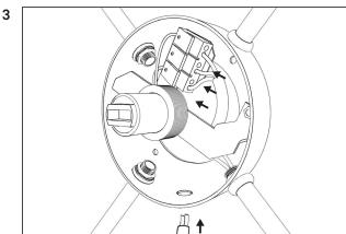
Lead the power cable in through the back or bottom of the where the cable connector resides.
