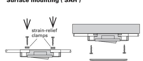
The strain-relief clamps must be screwed into the back of the switch housing as shown in the diagram.
