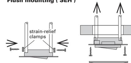
The strain-relief clamps must be screwed on the sides as shown in the diagram.
