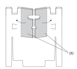
2. Open the bulkhead doors (B) and carefully remove it from the lamp. Do the same with all bulkheads.
