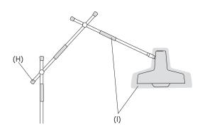
5. Remove rubber pads and plastic bags (I) left behind. Also, remove plastic caps (H) protecting the end of each arm.
