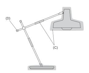
3. Remove rubber pads and plastic bags (C). Also, remove plastic caps (D) protecting the end of each arm.
