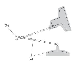
3. Remove rubber pads and plastic bags (C). Also, remove plastic caps (D) protecting the end of each arm.
