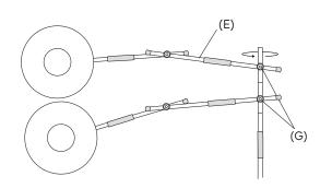
Rotate upper arm 180 degrees counterclockwise around the base. Ensure all the screws on the arm joints (G) are facing the same side.
