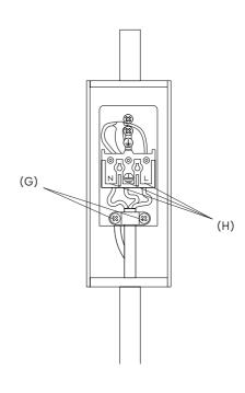
Unscrew the two screws (G) from the back of the lamp housing. Press N, ⊕, L tabs, (H) on terminal strip to pull the cable out.
