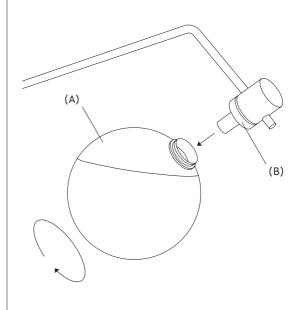
1. Unscrew the diffuser (a) while holding the metal ring (B).
