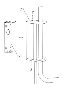
2. Remove the wall mounting (D) by unscrewing two screws from the lamp body (C).
