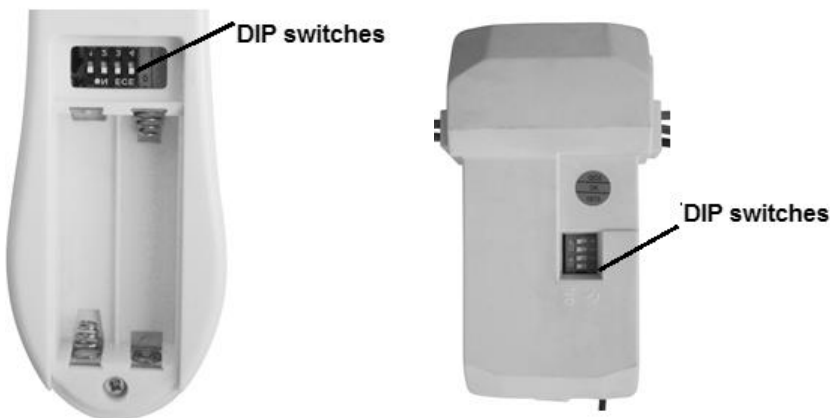
Fig. 11 Remote battery compartment
