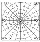
Luminous flux luminaire 551 lm
