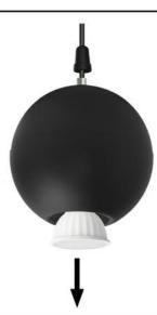
2. When the nipple is unscrewed the GU10 bulb, with the socket, will slide out of the lampshade.
