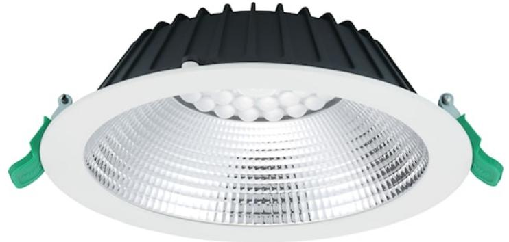
Insaver is a ceiling recessed LED downlight (IP44 from the front), Die-cast aluminium body, loop in loop out connector for quick installation, Dimmable DALI driver of TRIDONIC (LCA 25W 350–1050mA one4all SR PRE 28000671), 20W; 2500lm; 125lm/W; 4000K; UGR <19 with shallow product depth 60mm. Meets TP(a) requirements.
