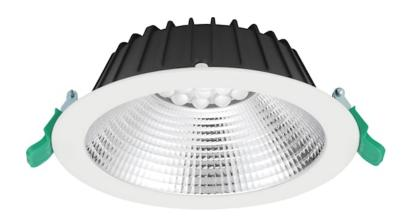
Insaver is a ceiling recessed LED downlight (IP44 from the front), Die-cast aluminium body, loop in loop out connector for quick installation, Non dimmable LED driver, 13W; 1700lm; 131lm/W; 4000K; UGR <19 with shallow product depth 60mm. Meets TP(a) requirements.
