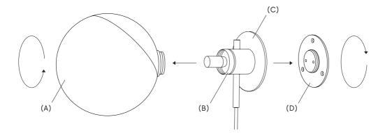
1. Unscrew the diffuser (A) while holding the metal ring (B). Unscrew the mounting plate (D) from the lamp body (C).
