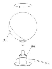
1. Unscrew the diffuser (A) while holding the metal ring (B).
