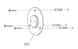
2. Mount the mounting plate to the wall with three appropriate screws and plugs. Always use correct screws and plugs for the mounting surface.
