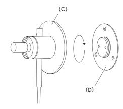
3. Attach the lamp body by screwing it onto the mounting plate. Make sure that cable is facing down.
