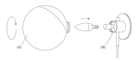
4. Insert the light bulb, then gently mount the diffuser screwing it back to the metal ring.
