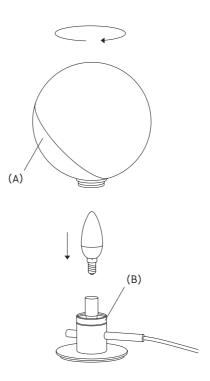
2. Insert the light bulb, then gently mount the diffuser screwing it back to the metal ring.
