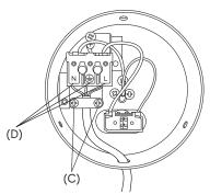
Unscrew the two screws (C) from the back of the lamp housing. Press N, (2), L tabs (D) on terminal strip to pull the cord out.
