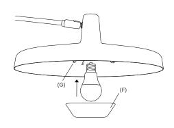
To insert the light bulb, release the undershade (F) by pressing three undershade brackets (G) inwards.
