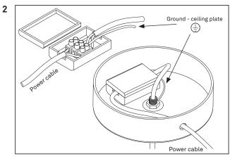
Install the power cable by either leading the cable through the top or the side of the ceiling plate and into the cable connector inside the connector box.
