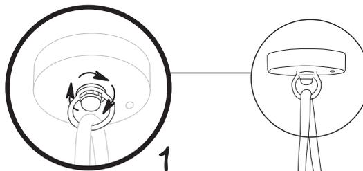
Slightly unscrew the nut and rotate the ring in order to adjust the position of the Monkey Lamp.
